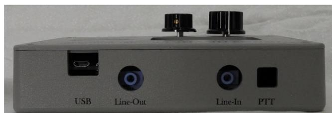
**Fig 5. Production Front Panel and side connections**
