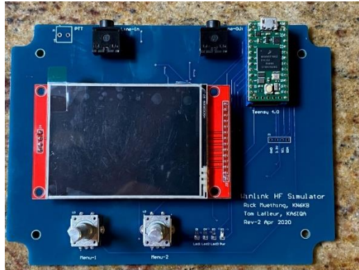
Fig 3. Basic control/display layout (Rev 2 prototype) Schematic, PCB design, layout assembly and test by Tom Lafleur KA6IQA
