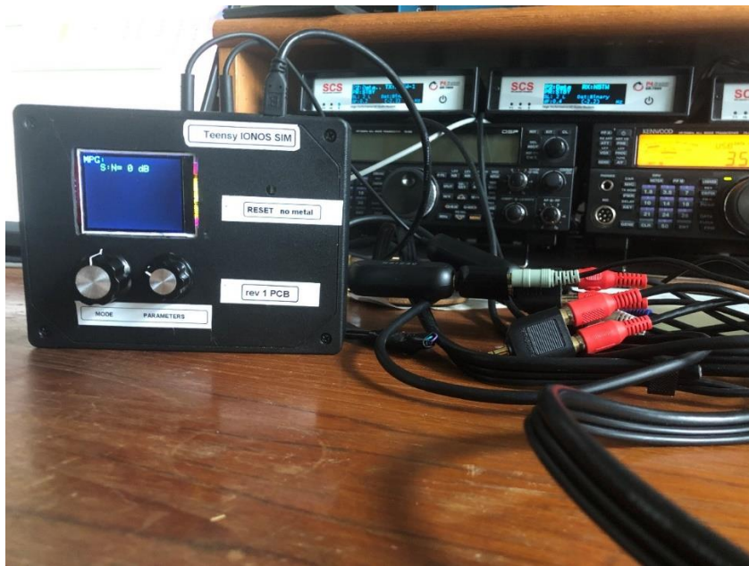
Figure 1 Test setup at N5TW using an early prototype IONOS Simulator
