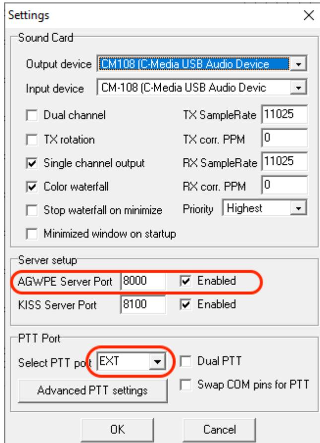
Select your sound card interface as the Input and Output devices. Enable the AGWPE port, use the default port number of 8000 (unless you have good reason to change it). For DRA type sound card devices, set the PTT Port to EXT.
