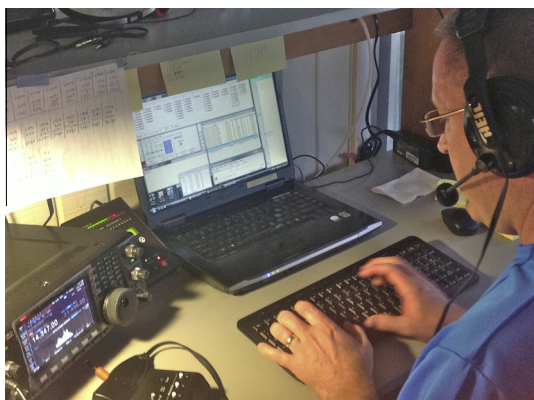
Fig. 1. This operating position is part of a health care professional's Amateur Radio station. The radio transceiver itself (lower left) uses digital technology for control and various stages of signal processing, much like a modern laboratory instrument. It can function independently, or be linked to a personal computer. Software exists for radio and antenna control, contact logging, shortwave propagation modeling, digital communication encoding and decoding, and passing message traffic to and from the Internet. Photo courtesy Dr. Scott Wright, Mayo Clinic cardiologist, used with permission.
